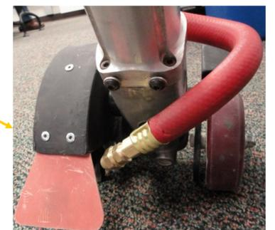
**Pneumatic Motor, Angle-adjustable air nozzle, and Debris Guard**
