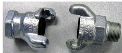
Simple Chicago fitting connection with existing air compressor
